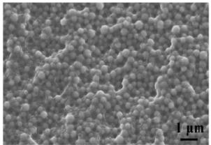
Figure 5. SEM image of silanized sample
